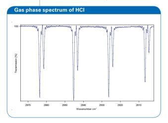
With its high resolution, the ALPHA is ideal for gas analysis. In the FTIR spectrum of the HCl the ro-vibrational lines are split due to the chlorine 35 and chlorine 37 natural isotopic ratio of 3:1.
