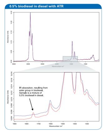
The high performance of the ALPHA results in short measurement times and low detection limits. Shown are the single reflection ATR spectra of diesel (blue) and 0.5% biodiesel in diesel after 60 sec measurement time.
