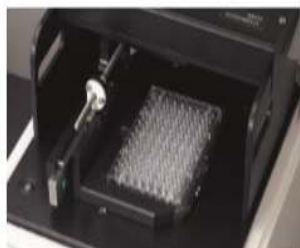
The Universal Platform Sampling accessory with Well-Plate
