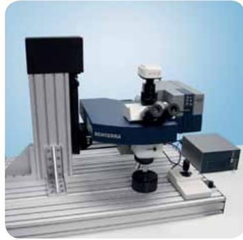
SENTERRA configured as an open architecture microscope.
