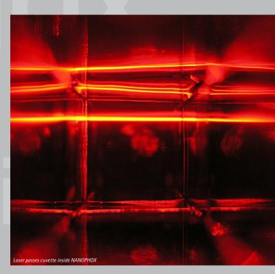
[3] viscosity and temperature remain unchanged, fine particles move faster than coarse particles. → Autocorrelation: The scattered signal is correlated with itself at different points in time (a comparison of the time lagged and the original function). • Multiple scattered light occurs if the incident laser light is scattered more than once by particles and disturbs the scattering wave on its way to the detector.
