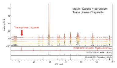
X-ray diffraction patterns from a three phase mixture of Chrysotile, Calcite, and Corundum. Patterns were collected on different mixtures down to 0.1 wt% of Chrysotile.
