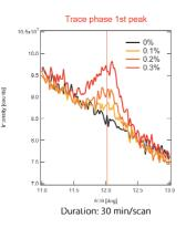
Zoomed area around the first small peak from the Chrysotile trace phase. In this case longer scans of 10 minutes show diffraction peaks visible above background down to 0.1 wt% Chrysotile.
